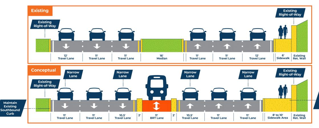
Widen Sidewalk Area In Front Of Retaining Wall
